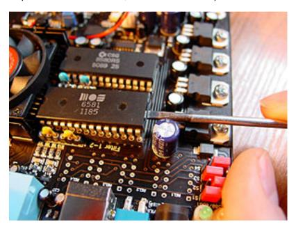
Step 4: Push the screwdriver further between the SID and the socket. Now that you have some place under the SID, you can push the screwdriver until almost the other end of the SID. The SID lifts a bit more so its pins are released from the socket at your end. The screwdriver's position is still horizontal.
