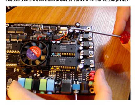
Step 2: Insert the tip of the screwdriver between the SID chip and the SID socket as shown on the picture. Don't push it further under the SID yet. Insert just the edge of the screwdriver's tip.
