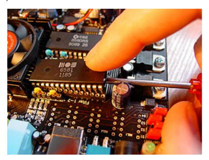
Step 5: Start pushing down the handle of the screwdriver carefully to lift the other end of the SID. Lift it until the SID gets horizontal. Now all pins of the SID are released from the socket.
