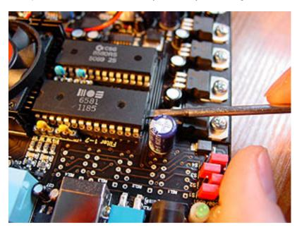
Step 3: Lift the SID a little bit, so the screwdriver's position will be almost horizontal.
