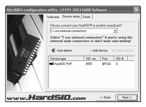
Click "Auto-detect" then click "Start" to re-detect the SID chip on the HardSID PCI, then click "Next" and "Finish".
