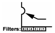
The SID needs two filter capacitors. There are three socket pins for both capacitors on the card. Pins 1-2-3 and pins 4-5-6 for the two filter capacitors.
